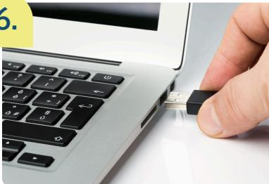
Plug the USB cable into the computer (USB-A socket).
