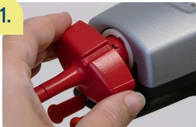
Insert the mouthpiece, paying attention to guide pin and guide slot.
