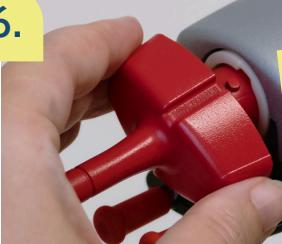
Insert the mouthpiece (note the guide pin and guide slot) and turn anti-clockwise with light pressure.
