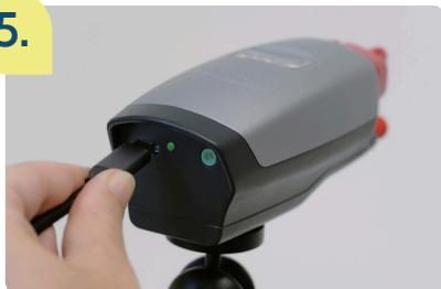
Plug the cable into the USB-C socket at the rear end of the IMAIR.
