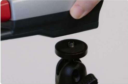
Illustration 7: Mounting the IntegraMouse AIR
